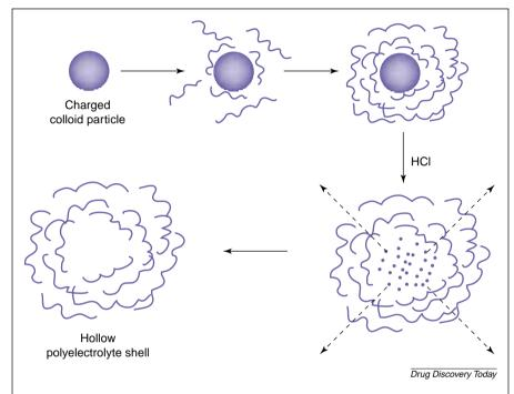
Figure 1. Producing a hollow polymer shell. Alternate layers of oppositely charged biopolymers are deposited onto a charged colloid particle until the required thickness is reached. On exposure to HCI, the colloid core dissolves and diffuses out to leave a hollow
